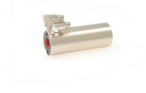
Artikel-Nr.: 0150-2708 PS10-70x80U-BL-QJ-D03 Stator 3x400VAC, Sin/Cos 1Vpp, KTY on power connector
