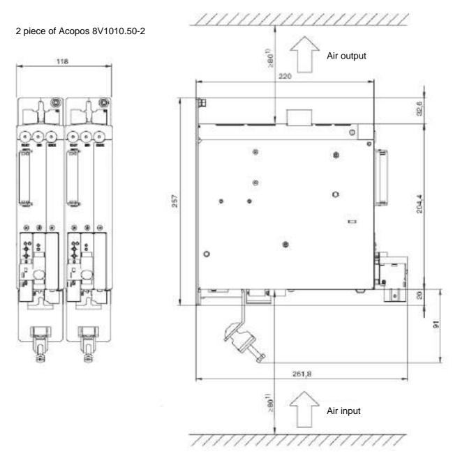
1) A free space of 80 mm must be provided above and below the ACOPOS drive to ensure adequate air circulation.
