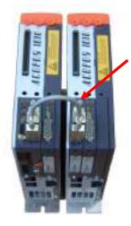
CAN-Adresses: Slot PLC: "0A" Plug-In Module AC110: "1B"
