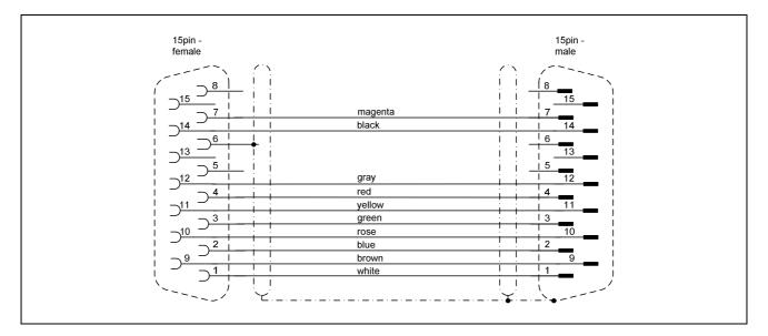
Red Marking = Feedback vertical motor Blue Marking = Feedback horizontal motor
