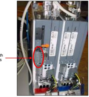
8-pin clamp with In- and Outputs
