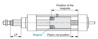
Figure 14: Position of the magnets.
