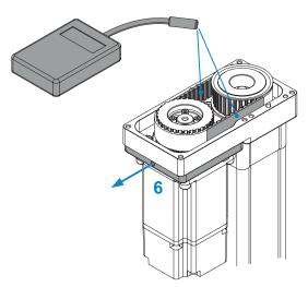
Figure 27: Belt pretensioning procedure.
