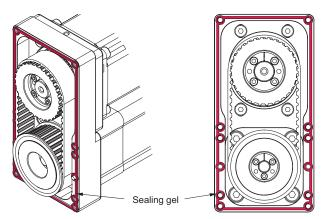
Figure 32: Sealing gel applied on the MSD housing **1**.
