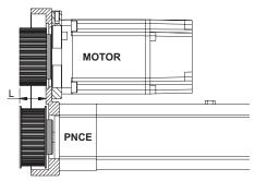
PNCE Т2 Туре T0 **T1 T**1 T1 T2 Gear ratio 1,5 1 1,5 1,5 1 1,5 1,5 2 2 1 1 Distance L [mm] 38.0 13.0 13.0 14.5 14.5 21.0 21.0 21.0 21.0 31.5 31.5 31.0 31.0 38.0 (± 0,2 mm) Belt pretensioning 235 185 215 190 320 320 215 225 250 190 215 225 155 155 frequency [Hz] (± 5 Hz)
