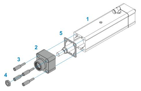
STEP 4: In the case of IP65 protection check if the seal of the PNCE 5, which is placed between the cylinder profile and the front cap, is damaged. If so, the seal of the PNCE 5 must be replaced with a new one.
