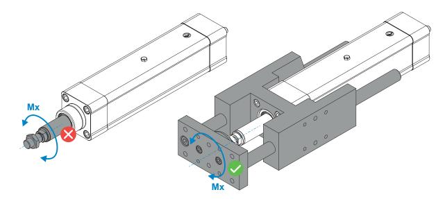
Figure 8: Piston rod subjected to torsional moment Mx.
