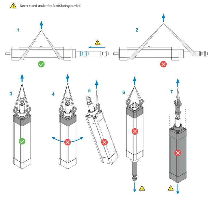
Figure 4: Carrying the electric cylinder.
