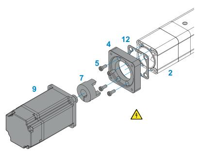
**STEP 4:** In the case of the IP65CR protection the seal of the motor flange **12** must be placed on the motor adapter housing **2**.
