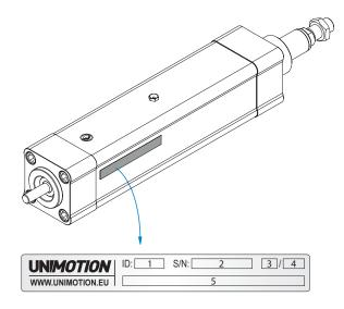
Figure 3: Identification label of the electric cylinder.
