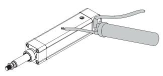
Figure 34: Lubrication of the ball screw drive.
