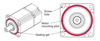
Figure 20: Sealing gel applied on the flange of the motor **9**.
