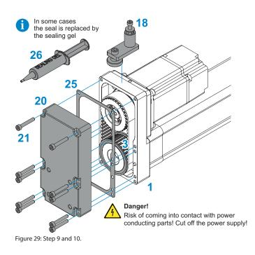
**STEP 9:** If the belt pretensioning unit was used, loosen the pretensioning screw **18** and remove the belt pretensioning unit. Slightly oil both flanges of the PNCE belt pulley **3** on the side where the belt is running on the pulley. Do not use the lubricant which cointains any solid parts!
