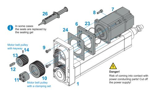
**STEP 3:** In the case of IP65CR protection the O ring seal of the motor **23** must be fitted on motor **7**. In some cases the O ring seal **23** is replaced by the sealing gel **26**. To use the sealing gel properly, please refer to the section **SEALING GEL** - Sealing the connection between motor and tensioning plate. Mount the motor **7** onto the tensioning plate **6** and tighten the screws of the motor **8**.
