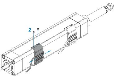
**STEP 3:** Adjust the sensor holder **1** together with the magnetic field sensor to the desired position. The positions of the magnets can be found in Table 3.
