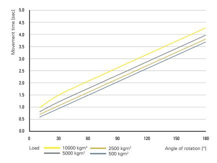
The mass moment of inertia of the aluminium rotary ring in standard dimensions is 111.7  $\mbox{kgm}^2.$
