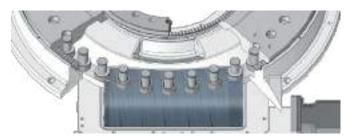
This cooling carousel at one of Cirex's casting stations in the Netherlands has a diameter of 10 metres and weighs 30 tonnes. It is driven by a CR. A special bearing has been fitted to handle the high tilting moment as a result of the uneven load.
