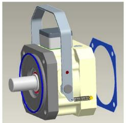
A **hand release lever** is available for the ROBA®-topstop® single circuit brake standard design as a special accessory. Please note that the hand release prevents the safety brake from functioning during operation. With hand release lever, only Protection IP54 possible. Size 200 (Type 899.\_\_\_\_2) hand release not possible.
