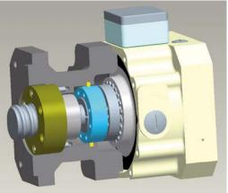
The ROBA®-topstop® single circuit brake with integrated ROBA®-ES shaft coupling is conceived for mounting onto a ball screw spindle. The special friction flange is adapted to the machine tool. The ball screw spindle bearing is integrated into this special flange, and at the same time serves as the friction surface for the brake. This compact construction is only minimally longer than a construction without the brake.
