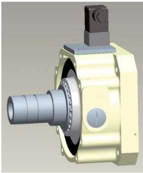
This ROBA®-topstop® single circuit brake is mounted directly onto a gearbox. The gearbox input side is adapted to the brake module interface. The special shaft bearing is located in the gearbox. It carries the input pinion. The ROBA®-ES shaft coupling is integrated into the brake module. The respective centering diameter and screw-on pitch circles for the servomotor are mounted in the housing flange.
