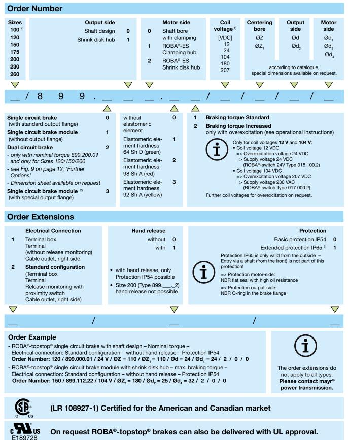
1) Permitted Voltage tolerance according to DIN IEC 60038: ±10 %
