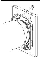
Optionally, there are two bore holes [N] on the gear housing for pinning the gearbox to the machine. You can fasten the gearbox to the machine with cylinder pins.
