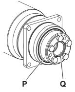
The slip-on shaft / hollow shaft / hollow shaft interface [Q] is axially secured to the load shaft by means of a shrink disk connection. If a gearbox with shrink disk [P] was ordered, then it is already mounted.
