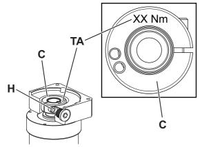
The tightening torque value [TA] of the clamping bolt [H] can be found on the clamping hub [C] and on the identification plate (optional).
