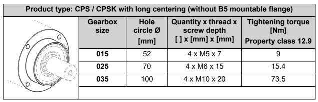
Tbl-24: Specifications for mounting to a machine CPS / CPSK with long centering
