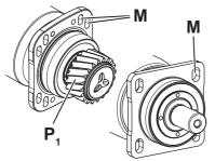
The gearbox can be optionally equipped with an output pinion  $[P_1]$ . The gearing backlash between output pinion and toothed rack/ counter-wheel can be adjusted using the slotted holes [M] and the lateral guides. An additional adjustment device is no longer necessary.
